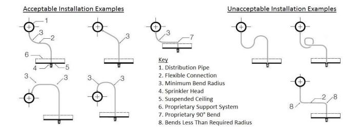
**Note:** Any damaged, kinked, or incorrectly installed flexible sprinkler connections, or any that have been adjusted in any way subsequent to the original installation must be stripped-out, scrapped, and replaced with new.
