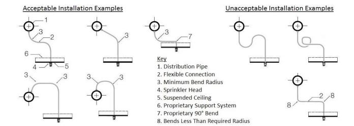
**Note:** Any damaged, kinked, or incorrectly installed flexible sprinkler connections, or any that have been adjusted in any way subsequent to the original installation must be stripped-out, scrapped, and replaced with new.
