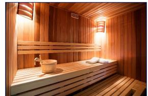
There are various types of saunas, but most commercial arrangements are typically constructed mainly of insulated timber; housing a heater, which is usually electrically operated and thermostatically controlled; with operating temperatures between 65C to 100C, at low humidity. As a result, there are numerous hazards, including potential hot surfaces and ignition sources with combustible loading in very close proximity.
