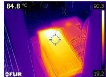
These risks should be assessed and can be easily verified using a thermal imaging camera. If dust can accumulate on these surfaces, it is prudent to select and install equipment whose external surfaces cannot reach the products Layer Ignition Temperature. The "T" Class of equipment which is
