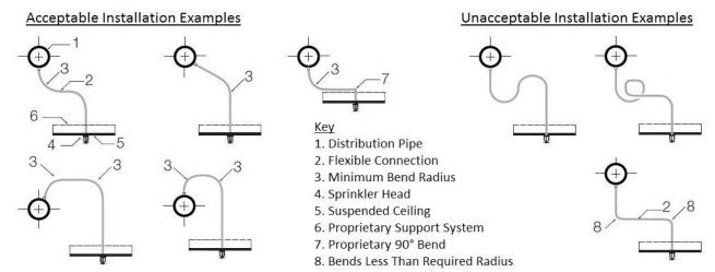
**Note:** Any damaged, kinked, or incorrectly installed flexible sprinkler connections, or any that have been adjusted in any way subsequent to the original installation must be stripped-out, scrapped, and replaced with new.
