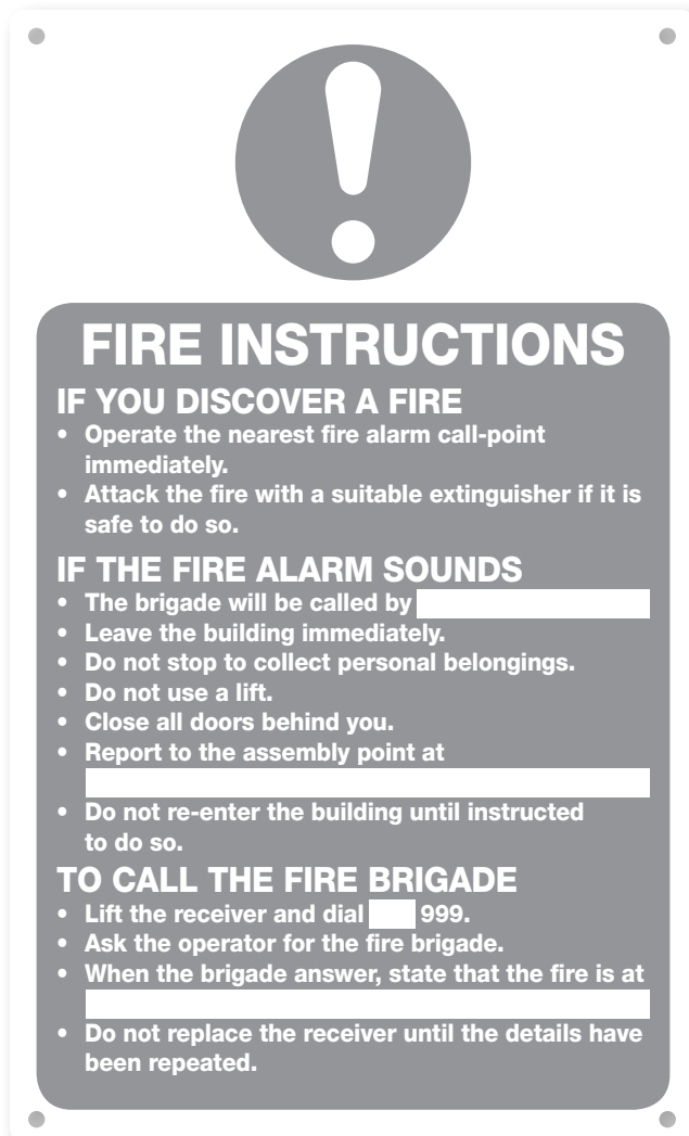
Figure 1: Typical fire action notice
