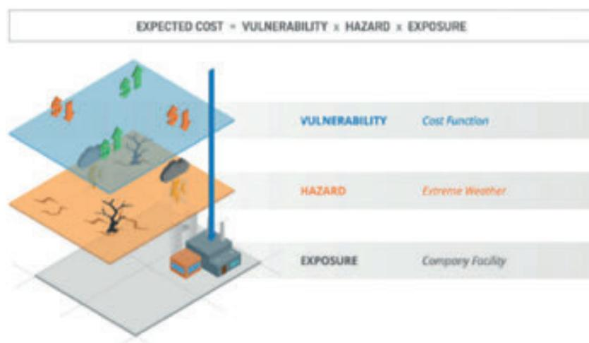
The cost (in figure 27) is built up by mapping the facilities onto a world map, with measures that define the facility's exposure to different extreme weather hazards, and then combining this with a vulnerability function that converts the exposure and an assessment of the physical hazard impact in each scenario into an estimated monetary cost, per facility.
